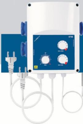
The GTEE1 fan speed controller automatically regulates the speed of single phase voltage controllable motors (230 VAC / 50–60 Hz) according to the measured temperature values and controls a heater according to a temperature setpoint. The fan speed will increase as the measured temperature exceeds the setpoint temperature.
